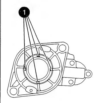
Checking drive-end bearing
